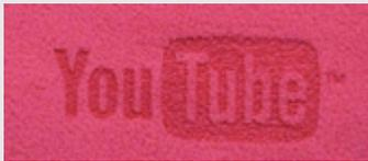
**Laser Etching:** A process that uses laser technology to etch or burn a mark on fabric.
